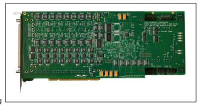
PCI TMS-320C6713 Floating Point DSP
