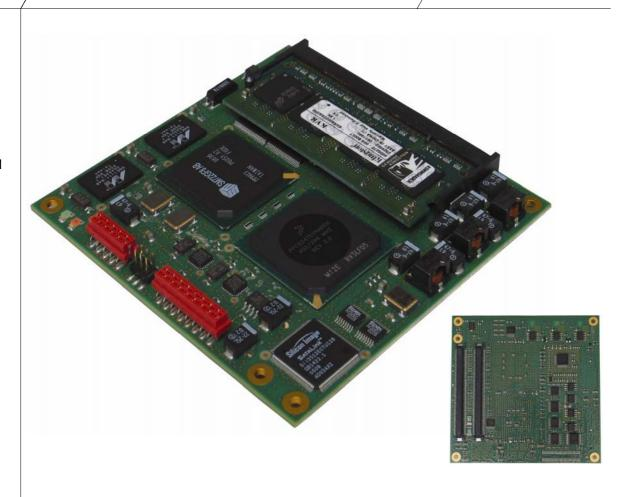
XCOM-9347 is a highly integrated solution specially designed to meet PICMG COM.0 standard requirements. It features a low-power high-performance PowerPC processor in COM Express Compact (microETXexpress) form factor, only 95x95 mm
