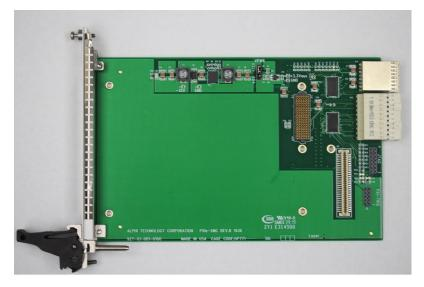
I/O and used to provide additional Ports controlled by the XMC. The added I/O ports are electrically controlled by the XMC module. The PXIe and PXI signals are routed to the FPGA via the user I/O J14 on the XMC.
